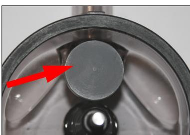
*The shut-off plug is made of silicone but not of rubber. It is larger than the plug in some other claws this is for a proper shut-off.*
