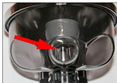
*The plug has a long spindle. This allows a good milk flow in the open position. Some claws have a plug with a shorter spindle*
