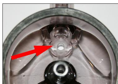
*The seat of the plug is machined in every claw bowl for a reliable shut-off. If the bowl is not machined the plug might not seal properly.*
